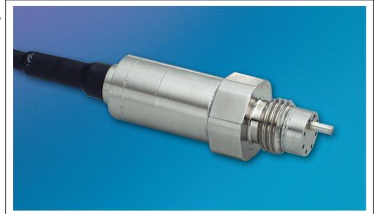
The ETLR/T-634-375 (M) is a miniature threaded redundant pressure transducer/platinum RTD combination. The two pressure transducers utilize a patented leadless technology. The platinum RTD protrudes beside the diaphragm to sense media temperature. The pressure and temperature devices are designed to operate independently. All wetted parts of the transducer are compatible with most industrial and automotive fluids.
